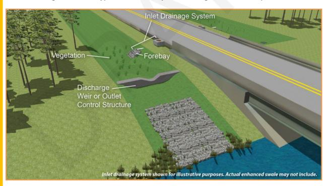
Figure 5.3-3 Typical Enhanced Wet Swale Configuration and Components
