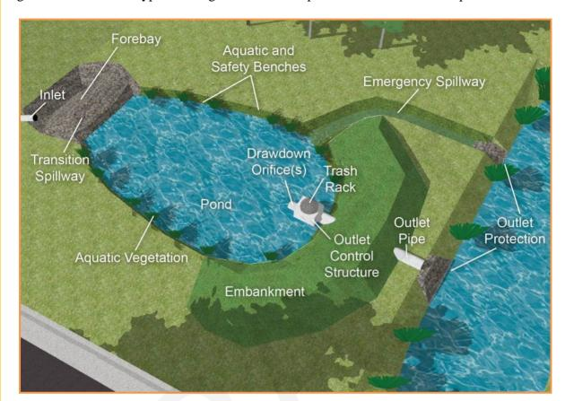
Figure 5.7-2 shows the typical configuration and components of a wet detention pond.
