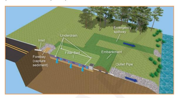
Figure 5.5-2 Typical Surface Sand Filter Configuration and Components
