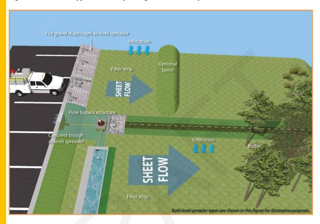
Figure 5.1-2 Typical Filter Strip Configuration and Components
