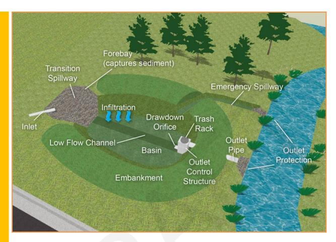
Figure 5.6-2 Typical Dry Detention Basin Configuration and Components
