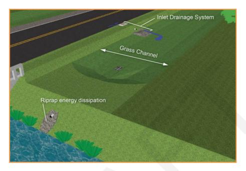
Figure 5.2-2 Typical Grass Channel Configuration and Components
