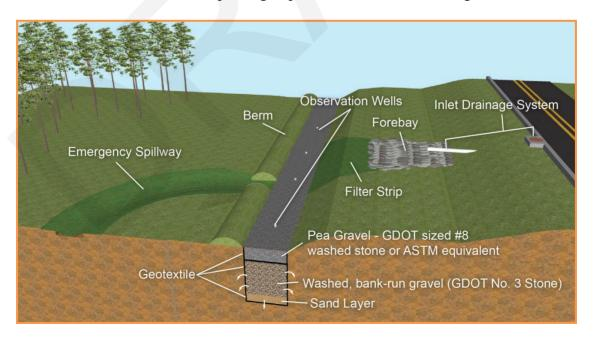
Figure 5.4-1 Typical Infiltration Trench Configuration and Components
