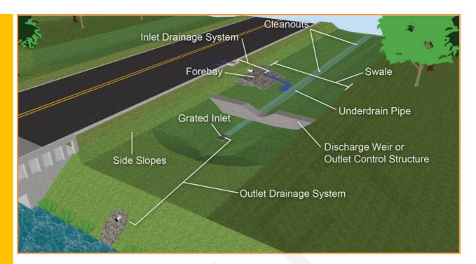
Figure 5.3-2 Typical Enhanced Dry Swale Configuration and Components
