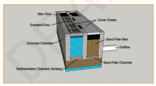
Figure 5.5-3 Typical Perimeter Sand Filter Configuration and Components
