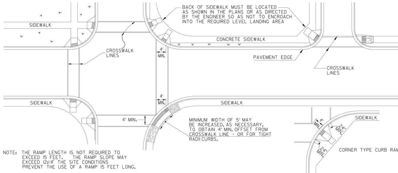
NOTE: THE RAMP LENGTH IS NOT REQUIRED TO EXCEED 15 FEET. THE RAMP SLOPE MAY EXCEED 12% IF THE SITE CONDITIONS PREVENT THE USE OF A RAMP 15 FEET LONG.
