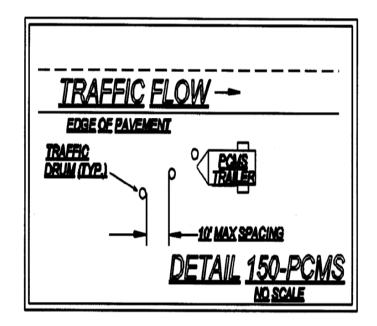
When not in use the PCMS shall be removed from the roadway unless protected by positive barrier protection. If the PCMS is protected by positive barrier protection the sign panel shall be turned away from traffic when not in use.
