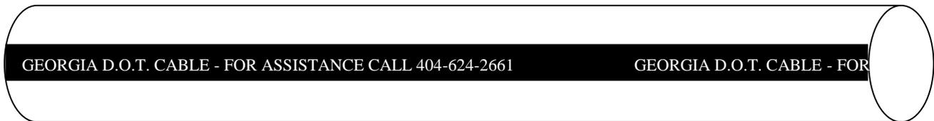
Any additional wording on the conduit, such as "this side up" or "this side down", shall be consistent with the installation orientation.
